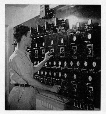
The control room is the brains of the new laboratory. Here, every possible climatic condition can be created.
