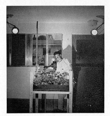
Photographic setup includes a prefocused camera, used to take pictures of all plants at regular intervals.
