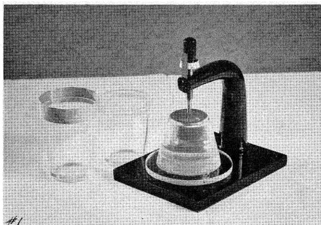
Ridgelmeter for the determination of jelly firmness.
