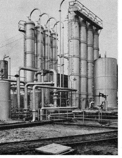
FIG. 1—Showing typical high-pressure absorber installation.
