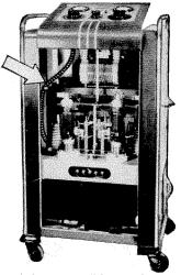
Here's how one well known electronic equipment manufacturer did it. The flexible shaft (arrow) connects control knob at top to a variable element at the bottom rear.
