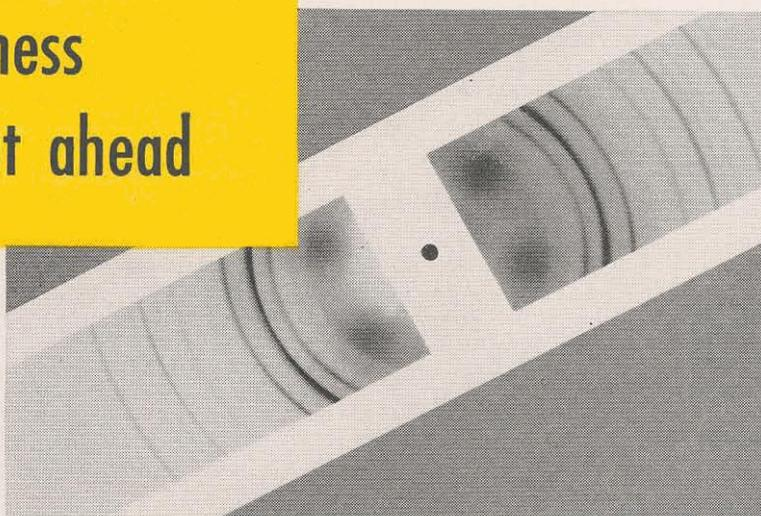
**REVEALS STRUCTURE AND CONDITION OF METALS**—X-ray diffraction patterns on Kodak films or plates provide important information concerning the crystal structure of metals. These patterns help show how alloys can be improved or new alloys made—give data on the effect of machining, drilling, and punching upon the structure of the material.
