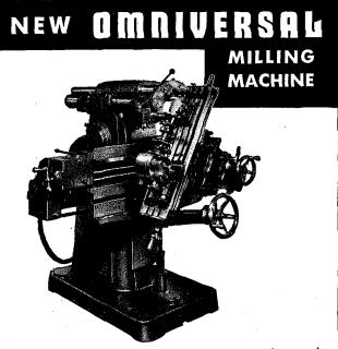
Designed for toolrooms, experimental and research laboratories the No. 0 Omniversal with swivelling knee and Omniversal Milling Head provides an easy and accurate means of obtaining both simple and compound angular settings of the work -- often permitting complete precision machining of a piece without relocating it in the holding device. Brown & Sharpe Mfg. Co., Providence 1, R. 1., U.S.A.
