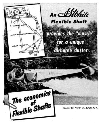
When the manufacturer of this crop-dusting helicopter wanted to transmit power from the accessory gear box to the insecticide pump, mounted some distance away, he chose an S.S.White flexible shaft to do the job. As the diagram shows, the shaft provides a simple one-piece coupling that can be readily run around intervening struts and frames.
