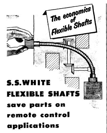
Just compare the simplicity of the flexible shaft control, shown above, with the combination of rods, bevel gears, pulleys and belts that might otherwise be necessary. The savings in parts and costs are obvious. What's more the flexible shaft is less complicated, needs no alignment; is easier to install and gives more freedom in mounting the coupled parts where desired to assure better and more convenient operation.
