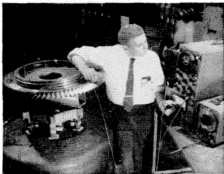
Instrumentation engineer at Pratt & Whitney Aircraft is shown investigating modes of vibration in a blade of a single stage of a jet engine compressor.
