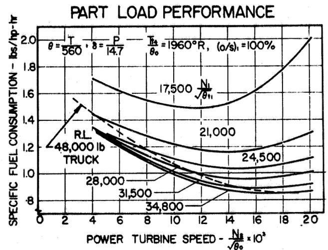
Fuel consumption vs power turbine speed. Turbine inlet temperature 1,500°F. (Ref. 12) (Ford)
