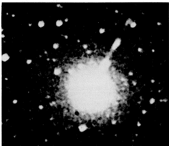
One of the ultrafast luminous pellets emerging from the flash of the coruscative explosion. In this photograph, made with a super Schmidt camera equipped with an interrupting shutter operated at 1800 cycles per minute, the distances between the interruptions of the track allow calculation of the speed of the pellet.
