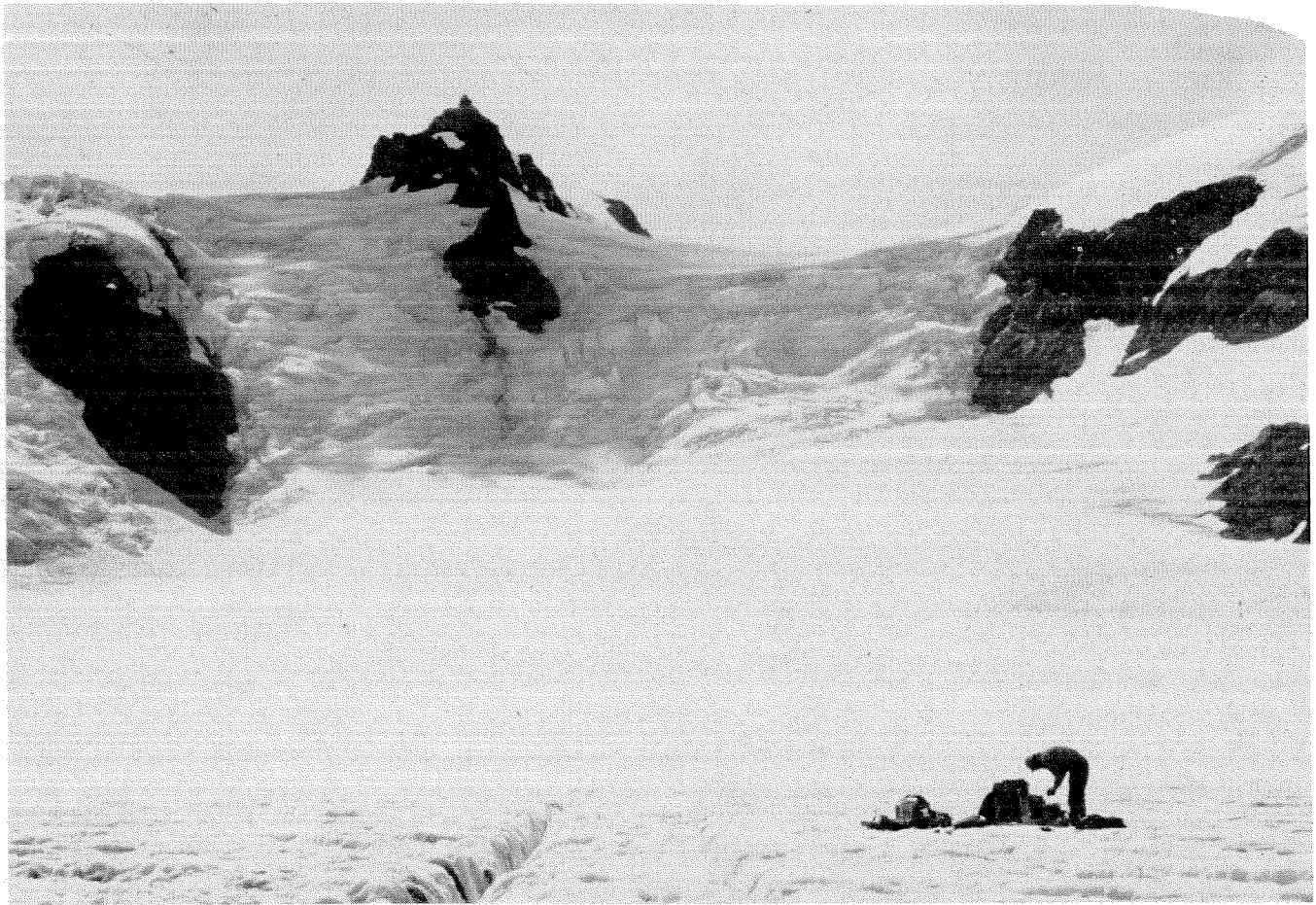
Clarence Allen, assistant professor of geology, gets ready to make a dynamite charge for seismic wave soundings. The depth of the glacier is exactly 910 feet.
