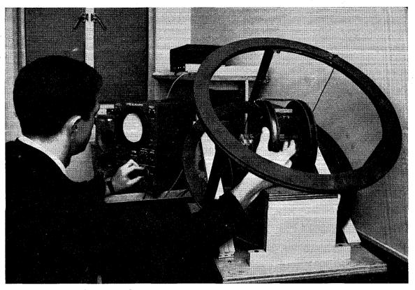
MAGNETIC FILM RESEARCH Magnetic properties of thin nickel-iron films are investigated with a "B-H Looper." These films can be used either as memory elements, or for switching logic circuits in a computer. They can be switched in only a few thousandths of a microsecond.
