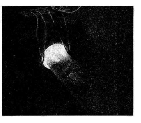
SOLID STATE TECHNOLOGY "Zone refining" is a technique especially developed to provide the high-purity materials needed in making solid state devices. The material to be purified is placed in an inert environment and repeatedly passed slowly through a furnace. Impurities accumulate in the molten zone, thus gradually increasing the purity of the resolidifying region. Figures like one impurity in 10<sup>10</sup> are now commonplace.
