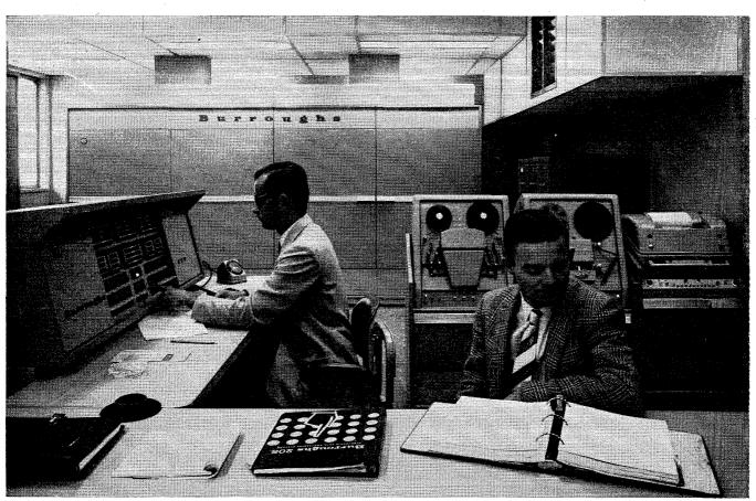
Large scale computers have become essential to modern science and technology. In Caltech's Computing Center, this Burroughs 220 Digital Computer serves as the Institute's computing facility for both general research and instruction in machine computing methods.
