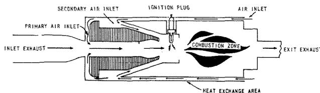
Two methods of controlling hydrocarbon emission from automobile tailpipes through combustion of the exhaust gases—a catalytic afterburner (left) and a direct-flame afterburner (right).
