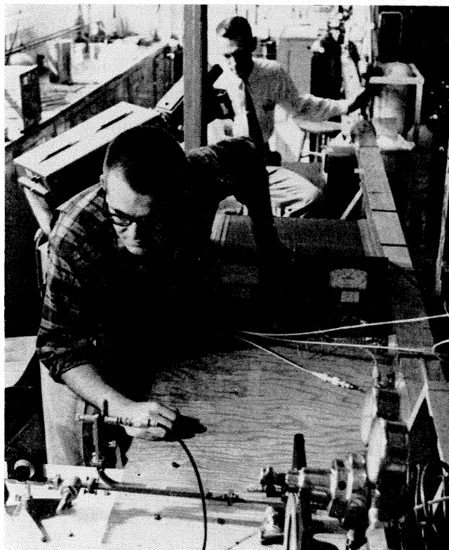
Kenneth Harwell, graduate assistant in aeronautics, and R. G. Jahn, associate professor of jet propulsion, use a 21-foot-long tube of argon to study the ionization of gases by shock waves. Conditions in the shock tube at high pressures are similar to those found in jet propulsion devices.
