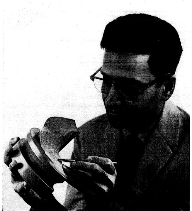
Sitaram Valluri, senior research fellow in aeronautics, in a practical demonstration of his new theory, studies the aluminum alloy hub of a large propeller blade that failed because of metal fatigue. The blade ripped
