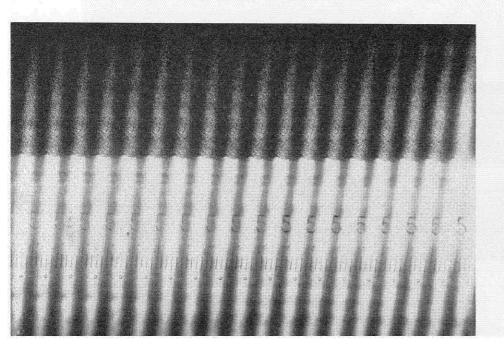
In high-speed photography, light intensity requirements are much more severe at greater magnification. This test photograph of a ground-glass microscope scale, magnified 25 times, shows the sharpness that can be achieved with the laser camera operating at 200,000 frames a second. Division marks on the scale are 100 microns apart.
