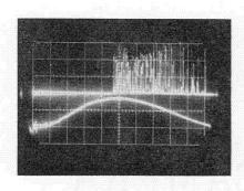
Left: Traces from a dual-beam oscilloscope show (lower trace) the intensity of the light entering a ruby laser and (upper trace) the random pulse intensities and timing of the light emitted by the ruby.
