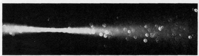
Vapor bubbles in water, generated by a focused laser beam. Magnified approximately 20 times.
