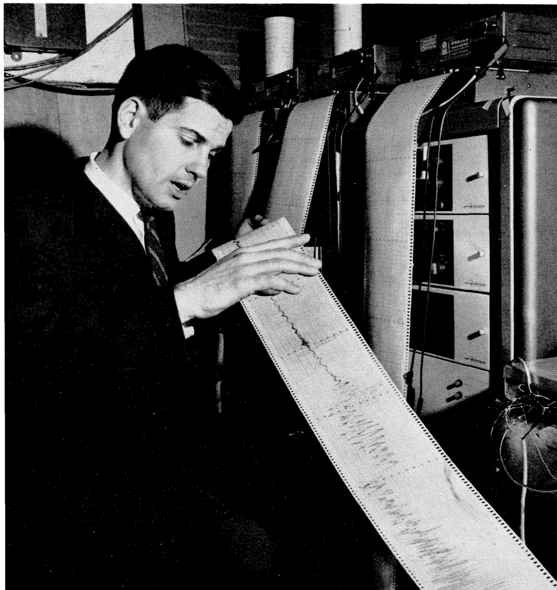
Stewart W. Smith, assistant professor of geophysics, examines a record of the Alaskan earthquake taken from an experimental, long-period seismograph that he is developing. This instrument differs from other seismometers in that it is especially designed for the very long-period vibrations of the earth, which can be likened to the ringing of a bell. It records directly on a magnetic tape that can be processed by a digital computer, where a type of spectrographic analysis is done that separates the various "tones" of the vibrating earth. This experimental instrument was put into operation only a few hours before the Alaskan earthquake.
