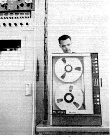
Research laboratories in the computing center use remote data transmission stations like this one to send data directly from the laboratory to the central computer system.
