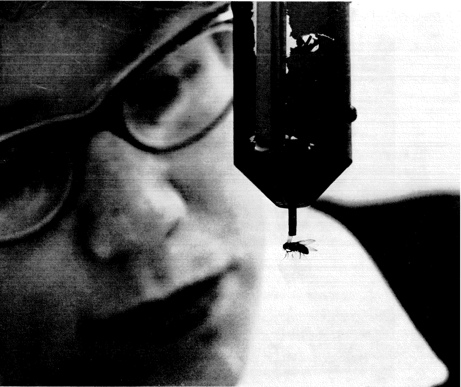
Housefly, attached to torque meter which measures wingbeat response as the fly tries to follow a visual target
