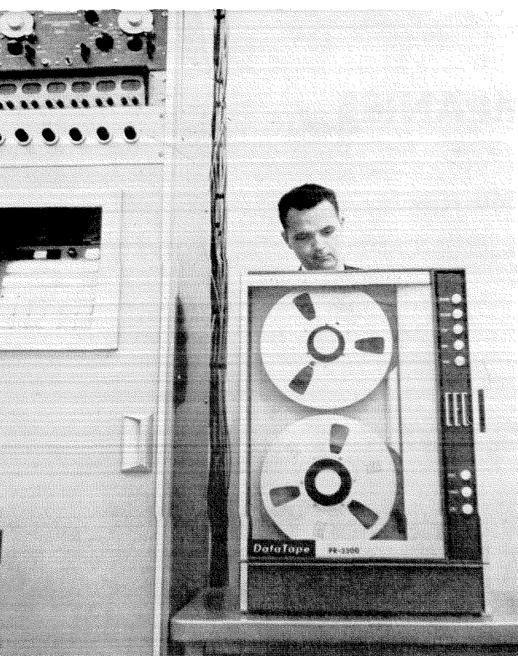
Research laboratories in the computing center use remote data transmission stations like this one to send data directly from the laboratory to the central computer system.
