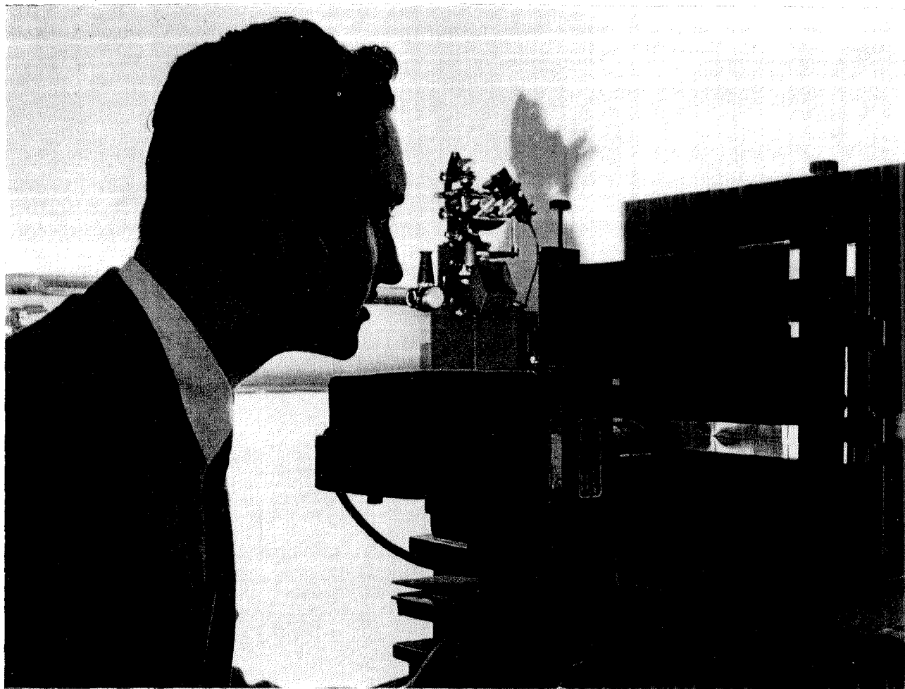
Wolfgang Knauss, research fellow in aeronautics, uses a sheet-straining device to measure the amount of energy that is dissipated when a fracture occurs in polymeric material.
