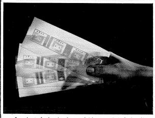
Laminated plastics for multi-layer printed circuits have to be a special breed—very thin, made to exacting tolerances, uniform, free of voids and pinholes, suitable for etching and all soldering operations.
