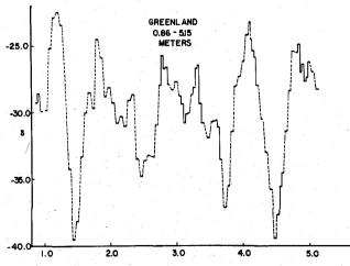
Seasonal effect observed in the  $O^{18}/O^{16}$  ratios in Greenland snow. The less negative values of  $\delta$  are for summer precipitation, and the most negative values are for the midwinter precipitation. The numbers on the abscissa represent the depth at which the samples are taken.
