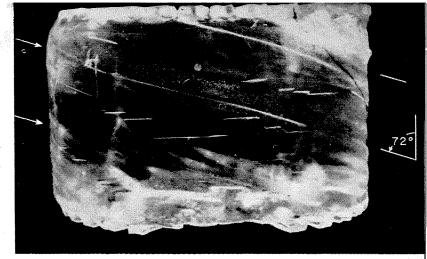
Highly sheared crystal of ice I. The sloping reference lines (arrows) were originally vertical, but were tilted through an angle of 72 degrees by plastic flow in the crystal, as shown. The total shear strain is 310 percent. The crystal is 8 cm in diameter.
