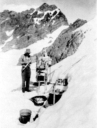
A drill site in the icefall. Barclay Kamb is preparing to lower the borehole camera to determine ice separation at the base of the glacier.
