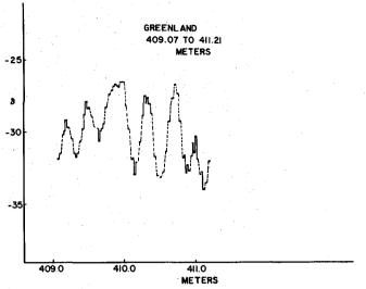
The variations with depth of the  $O^{18}/O^{16}$  ratios of Greenland ice taken from a depth ranging from 409.07 to 411.21 meters.
