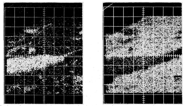
In the electron beam scans for K (left) and Na (right), the density of white spots is proportional to their concentration. The area shown, 85 microns on a side, is the same as the shaded area in the photomicrograph on the opposite page.
