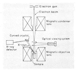
The basic elements of the electron microprobe x-ray analyzer shown in schematic form.
