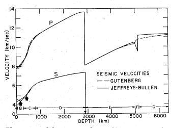
The major subdivisions of the earth's interior are determined from variations in the velocity of compression waves traveling through the earth: (B) upper mantle; (C) transition region; (D) lower mantle; (E) liquid outer core; (F) transition region; (G) solid outer core.
