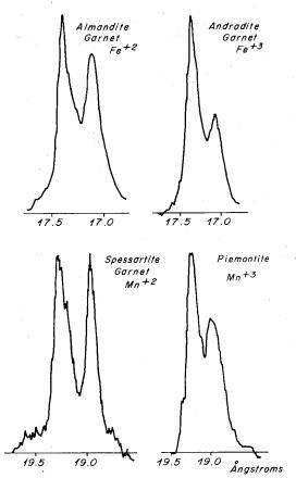
Portions of wavelength scans showing  $L\beta/L\alpha$  intensity for different minerals high in Fe<sup>+2</sup>, Fe<sup>+3</sup>, Mn<sup>+2</sup>, or Mn<sup>+3</sup>.
