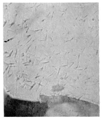
Fission tracks in a crystal of the mineral diopside from the Four Corners meteorite. The tracks presumably arise from the spontaneous fission decay of the nowextinct Pu<sup>244</sup>. The number of tracks shown corresponds to a density of 6,000,000 tracks per square cm. The dimensions of the picture are roughly 40 by 50 microns.
