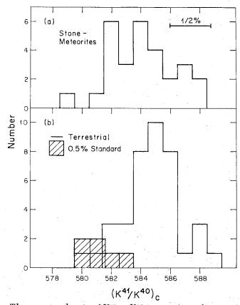
The measured ratio of  $K^{41}$  to  $K^{40}$  in a variety of meteoritic (a) and terrestrial (b) samples. No distinction in the  $K^{41}/K^{40}$  ratios in the two types of material could be detected. The sensitivity of the mass spectrometric measurements is shown by the cross-hatched squares, which are measurements of a standard which was enriched in  $K^{40}$  by 0.5%. (Measurements made in collaboration with H. J. Lippolt and G. J. Wasserburg.)
