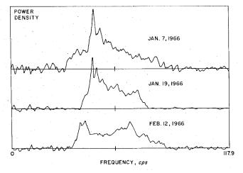
When a spectrogram is depolarized, topographic features can be seen clearly. In this series, peaks move from right to left, corresponding to Venus' rotation.
