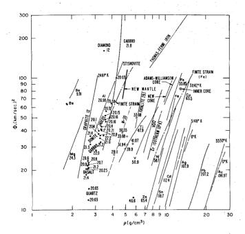
A comparison of laboratory shock wave data for rocks and seismic data (where  $\phi$  is the square of the hydrodynamic sound velocity and  $\rho$  is density) shows that the mantle has a mean atomic weight near 23 and that the core is slightly less dense than pure iron.
