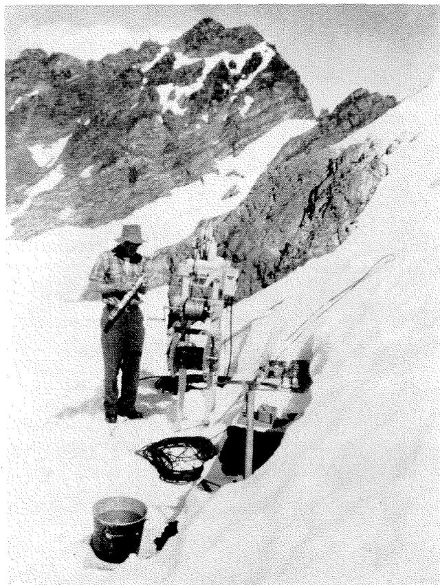
*A drill site in the icefall. Barclay Kamb is preparing to lower the borehole camera to determine ice separation at the base of the glacier.*
