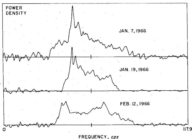
When a spectrogram is depolarized, topographic features can be seen clearly. In this series, peaks move from right to left, corresponding to Venus' rotation.
