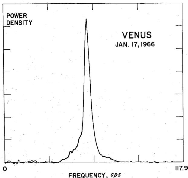
Radar spectrogram of Venus, made on January 17, 1966, shows that Venus is smooth to radio waves and would appear as a disk with a bright highlight at the center.
