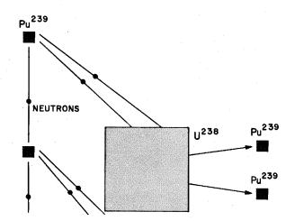
The plutonium fast breeder, the electrical power producer of the future, uses a costly fission energy fuel  $(Pu^{239} \text{ at } \$40 \text{ a gram})$ , but it will actually produce more  $Pu^{239}$  than it uses. Neutrons given off from the fission of one unit of  $Pu^{239}$  will not only keep the energy-producing chain reaction going, but, when combined with uranium 238, will produce two new units of  $Pu^{239}$ .
