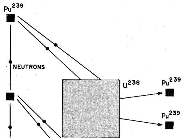
*The plutonium fast breeder, the electrical power producer of the future, uses a costly fission energy fuel ( $Pu^{239}$  at \$40 a gram), but it will actually produce more  $Pu^{239}$  than it uses. Neutrons given off from the fission of one unit of  $Pu^{239}$  will not only keep the energy-producing chain reaction going, but, when combined with uranium 238, will produce two new units of  $Pu^{239}$ .*
