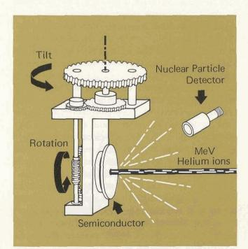
Schematic view of an experimental setup for determination of the lattice location of impurity atoms in a semiconductor. When the incident beam of helium ions strikes the sample, a small fraction are scattered back into the detector. The number and energy of these backscattered particles are measured as a function of sample tilt and rotation.
