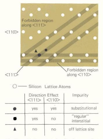
The diamond lattice typical of semiconductors, such as silicon, provides a simple case for determining the lattice location of impurity atoms. Well-channeled energetic ions do not penetrate into the lattice rows (forbidden regions) and cannot interact with impurity atoms contained within these regions. Consequently, one may determine the lattice location of the impurities from directional effects in the yield of backscattered particles.
