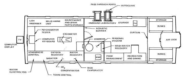
The floor plan of the 40-foot-long "home" for the four crewmen is a testimonial to careful planning and ingenuity in stowing a large amount of equipment into a compact area.
