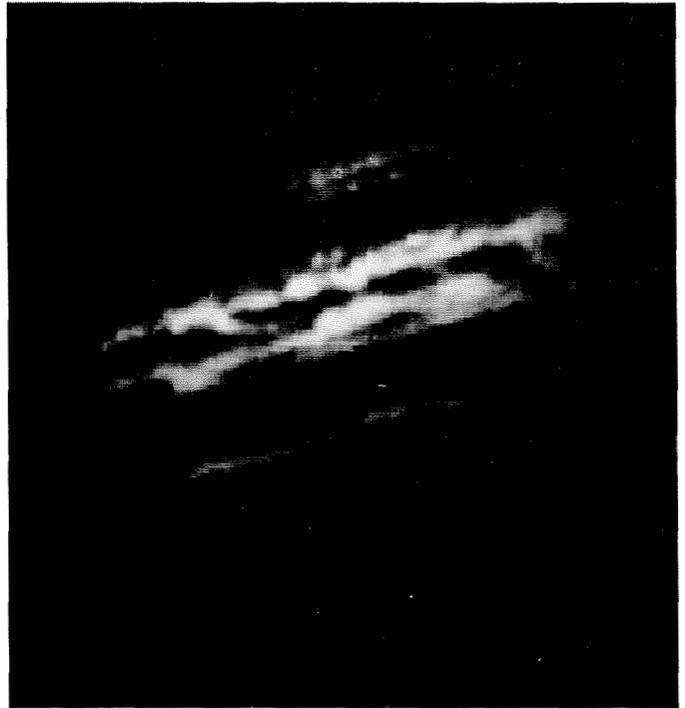
With the “wobbling secondary” and the new photocell, we were able to make a picture every 168 seconds, with a sharpness limited only by the turbulence in the earth’s atmosphere. Since last fall we have collected over 500 of these pictures along with occasional Kodachrome color pictures to compare the visible features with the 5-micron pictures, as in the examples above.
