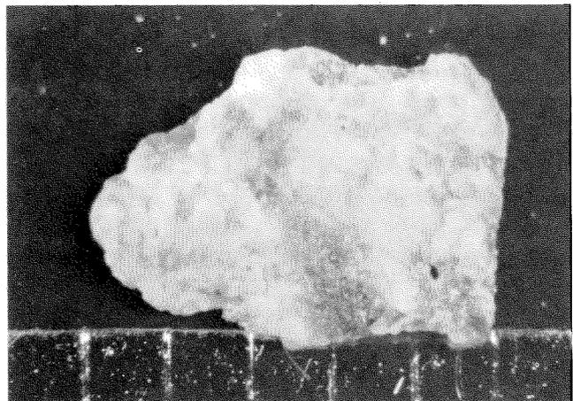
Lined up against a millimeter scale, a piece of lunar anorthosite measures just about 2½ millimeters — about half the size of a grain of rice. This is the larger of the two Luna 20 rock samples, each of which has now undergone analysis and age-dating procedures by a consortium of scientists at Caltech, Oregon State University, and the University of Chicago.
