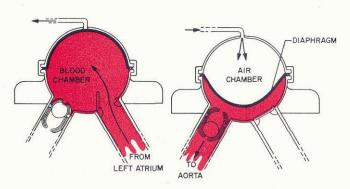
A schematic diagram of an artificial heart, designed to carry part of the pumping load for a period of days after a patient has undergone heart surgery. The diagram on the left shows the heart as blood is drawn in, and the one on the right as it is pumped into the aorta.
