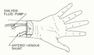
Artificial kidney of the future, as envisioned by Dr. L. W. Bluemle, Jr., of the University of Pennsylvania. The device would work continuously as part of the arteriovenous shunt using dialyzing fluid from a reservoir located on the patient's body.
