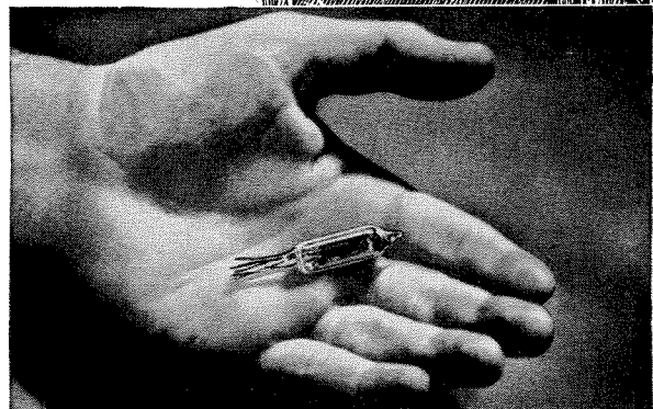
Typical Sylvania subminiature tube 1¼" long, pencil thin—heart of vital electronic equipment.
