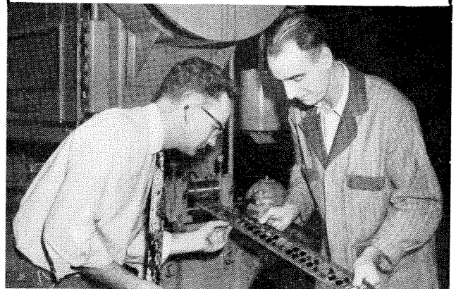
• Engineer and punch press operator check production of parts for newly designed grasshopper fuse.
