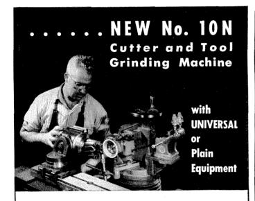
The new super-versatile No. 10N with Universal Equipment is especially designed for rapid, accurate toolroom work — light external and internal cylindrical grinding, surface grinding, as well as routine
