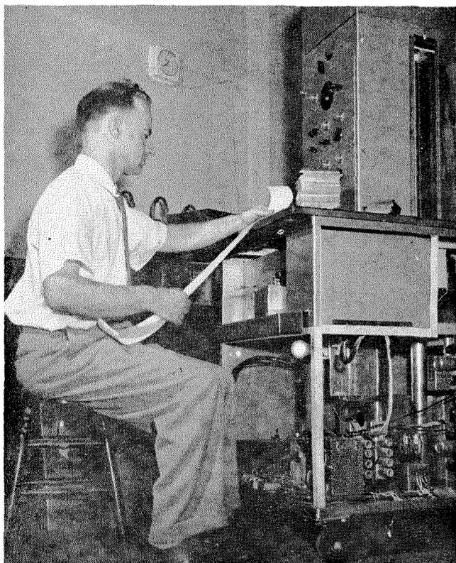
*Dr. Geoffrey Keighley's automatic counter measures minute radiation emitted by various materials resulting from "tagged atom" research. Samples move beneath a counting tube, which records reactions. These are transferred to a paper tape which can be read by the operator. The machine is currently being used to "count" radioactive samples obtained in a study of protein synthesis in the Institute's Biology Division.*
