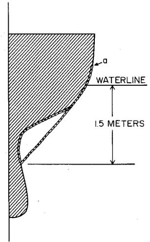
Figure 4: The chain midgirth measurement is the difference in length between a chain running from point "a" along the hull to a point 1.5 meters below the waterline and a chain stretched tight between those points.
