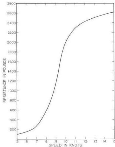
figures, levels off as indicated in Figure 10. Although sails cannot provide the several thousand pounds of thrust to cause a hull to plane, ocean waves frequently have slopes of 20 percent or more, and for a 24,000-lb. yacht, this gives a forward thrust of 4,800 lbs. or more — quite enough to cause it to plane.
