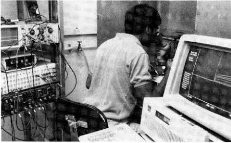
**Above: Measuring an individual cell's conductivity is exacting work. A microelectrode is inserted into the cell, using the microscope to guide the hand. Conductivity profiles appear on the computer monitor at right.**
