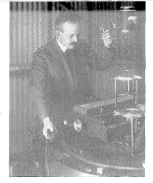
Right: George Ellery Hale uses his spectrohelicgraph in the Hale Solar Laboratory. Below: The 100-inch and 60-inch telescopes nestle side by side on Mount Wilson.
