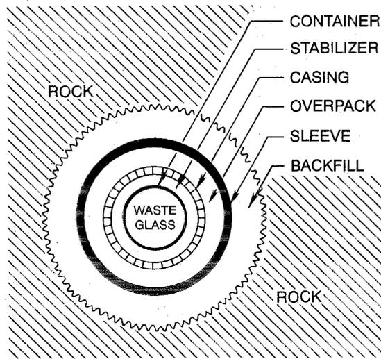
can probably be made to last several centuries. Around that is a stabilizer, which is there to stabilize physical and chemical properties. And around this there is another casing—and that is the real safety—made of some very resistant material, such as copper, as has been proposed by the Swedes. Then comes something called “overpack.” You now have this cylinder of material, which is let down deep into the earth and shoved into a tunnel.
