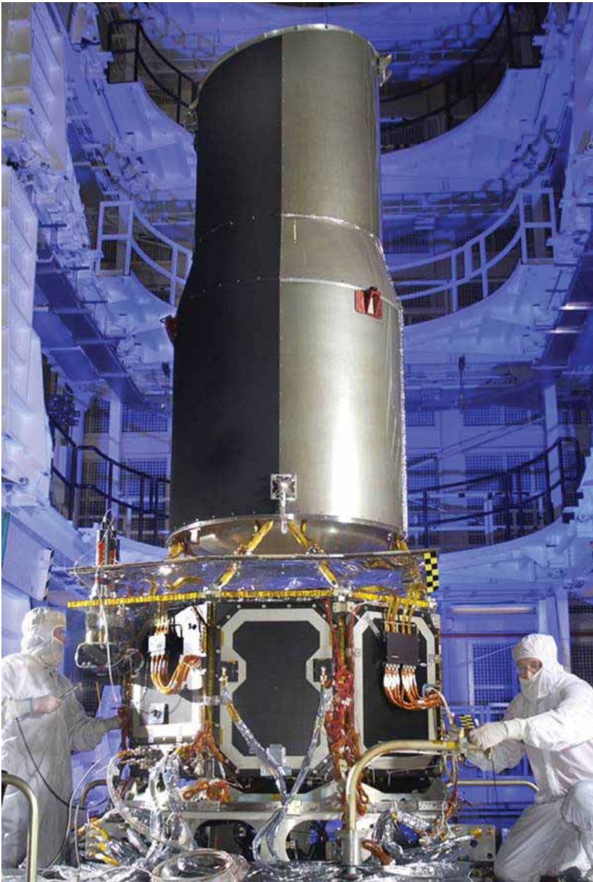
Above: Spitzer undergoing final assembly at Lockheed Martin's plant in Sunnyvale, California in 2002. The solar panel, which runs the length of the spacecraft down its shiny side, is not yet in place. The telescope proper fits into the narrow upper part of the barrel, which also contains two more heat shields. The cryostat lives in the bulge in the lower part of the barrel. The eight-sided box below the barrel contains the instruments' electronics, the power systems, and the equipment that aims the telescope and communicates with Earth, and is the only warm part. Above, right: Spitzer's location on November 24, 2003. The spacecraft is now over 8,000,000 kilometers away. An AU, or Astronomical Unit, is the mean distance from Earth to the sun, or 149.6 million kilometers.
