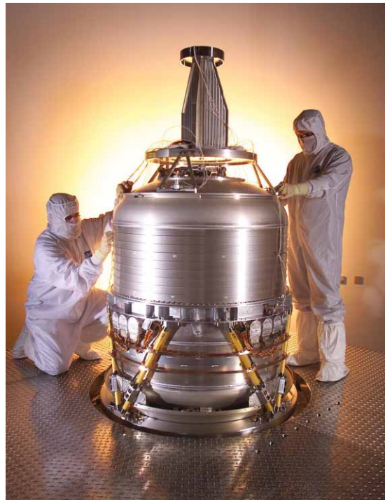
Below: Not frat boys praying to the beer god, but technicians mounting a mock-up of the telescope on the cryostat for a vibration test. The cryostat's rounded top houses the Multi-Instrument Chamber, which is only 20 centimeters, or about two handsbreadths, high. The helium tank fills the rest of the keg.
