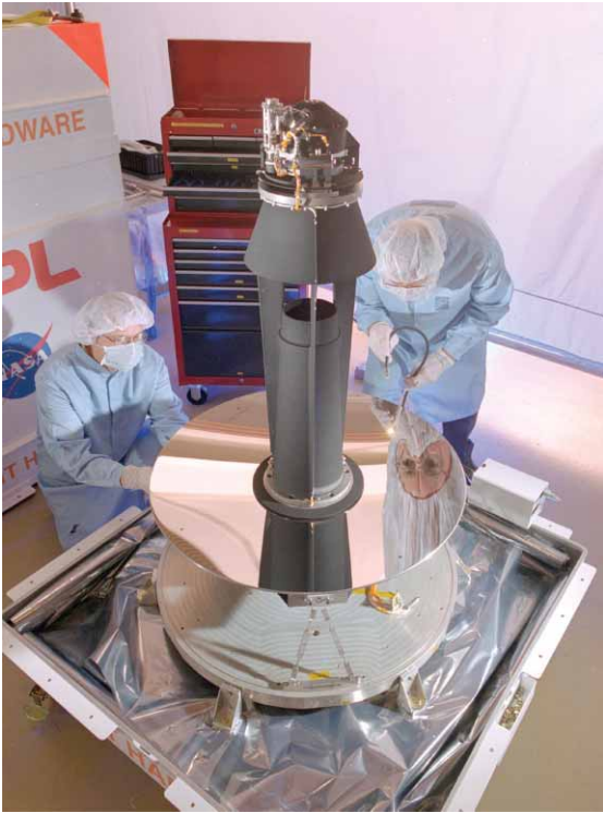
Below: Not frat boys praying to the beer god, but technicians mounting a mock-up of the telescope on the cryostat for a vibration test. The cryostat's rounded top houses the Multi-Instrument Chamber, which is only 20 centimeters, or about two handsbreadths, high. The helium tank fills the rest of the keg.
