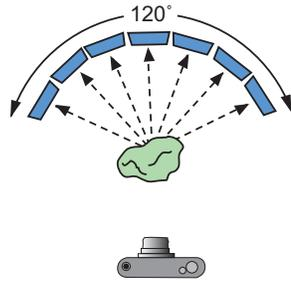
Doing tomography along one arc gives a set of pictures (blue) that don't show the subject from all angles, leading to distortions in the 3-D reconstruction in the wedge where data is missing. Rotating the sample 90 degrees and repeating the scan gives a second set of pictures (pink) that doesn't provide complete coverage either, but fusing the two sets (purple sphere) covers most points of view.
