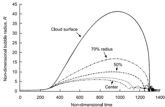
**When  $\beta$  is small, the collapse begins at the center and moves outward, causing the pressure front to dissipate.**
