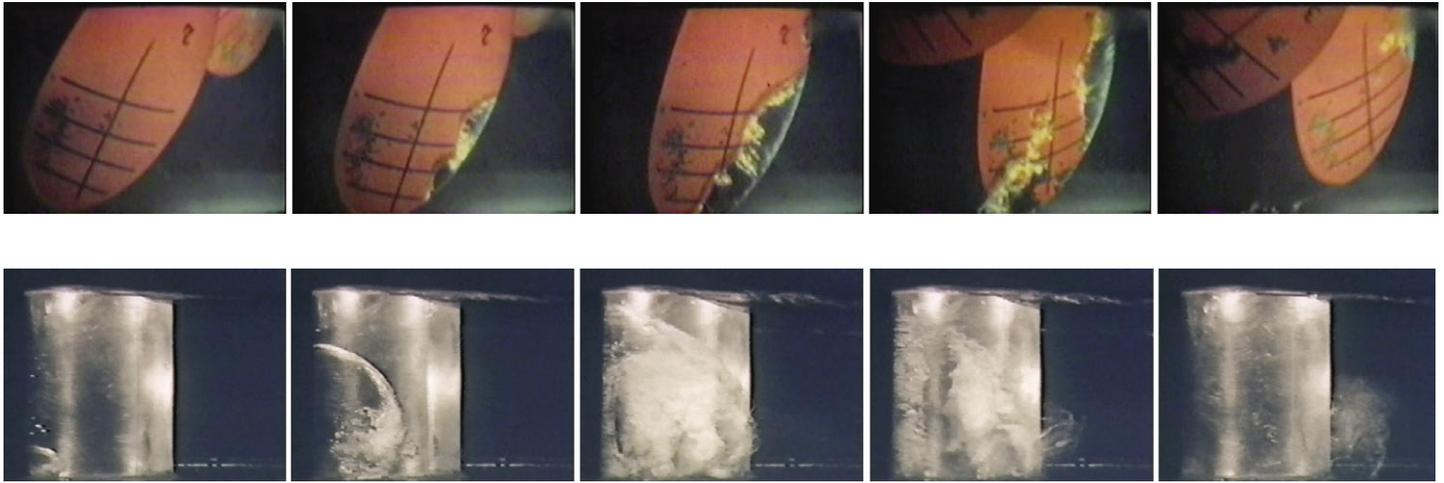
**Top:** The places where the paint was eaten off these propeller blades coincided with where the white clouds of bubbles were collapsing.
