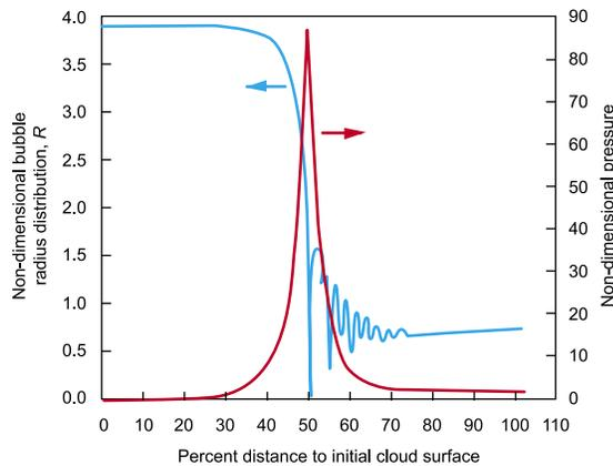
**The blue plot shows the bubbles' size (again, for  $\beta$  greater than one) versus their distance from the cloud center at the midpoint of the collapse process. The red curve is the pressure spike associated with the collapse.**
