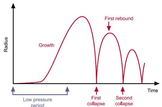
When a bubble collapses near a solid surface, the water has a hard time filling the void from the wall side. The collapse, initially symmetrical, becomes directed toward the wall, and a reentrant jet develops.
