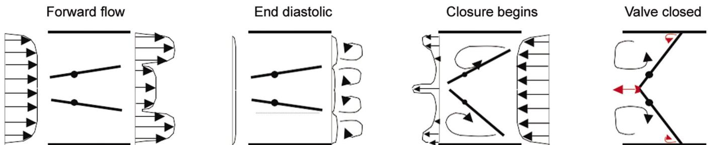
A bileaflet valve is a pair of flat plates mounted on off-center pivots. A reversing flow pushes the plates shut automatically, but also causes high-pressure jets (red) to shoot through the narrowing cracks in the final moments of closure.
