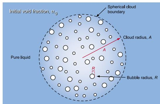
**A cloud of bubbles has three important parameters—its radius,  $A$ ; the average radius of its bubbles,  $R$ ; and the proportion of the cloud's volume taken up by the bubbles,  $\alpha$ .**
