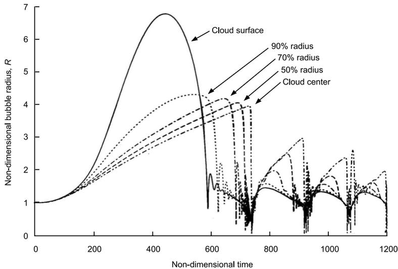
**Above: How bubbles grow and collapse at various depths within a cloud that has a  $\beta$  greater than one. The bubbles on the outside collapse first, creating an imploding pressure wave.**
