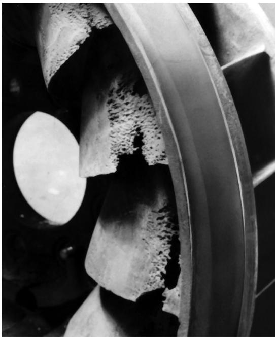
**Top:** The three pitted regions on the undersides of these blades are the early signs of cavitation damage.
