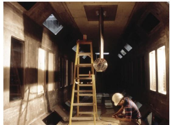
**The 10-inch headform being installed in the Large Cavitation Channel's working section.**
