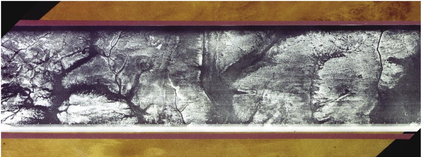
**This 50-kilometer-wide strip of SIR-A data, superimposed on a Landsat simulated true-color mosaic of the Sahara, shows ancient river beds buried beneath the sand.**
