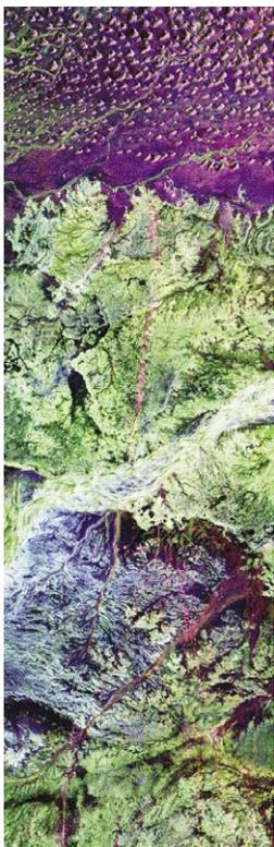
In this SIR-C image, sand dunes are magenta and limestone is green. "Ubar" sits just above the dry wash (light band) at center. Many tracks (red streaks), both ancient and modern, converge on the site from the south, but only one leads out into the desert to the north.
