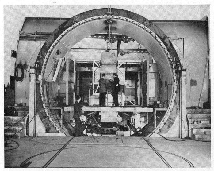
FIG. 15. Entrance to decompression sphere showing model cart in working section.
