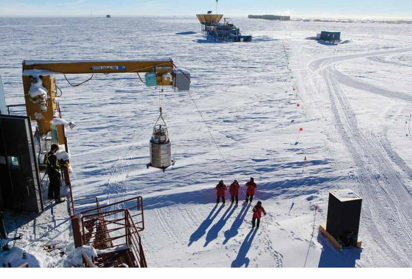
BICEP2 team members lift a liquid helium cryostat to the second floor of the Dark Sector Laboratory to chill the telescope to a temperature near absolute zero.
