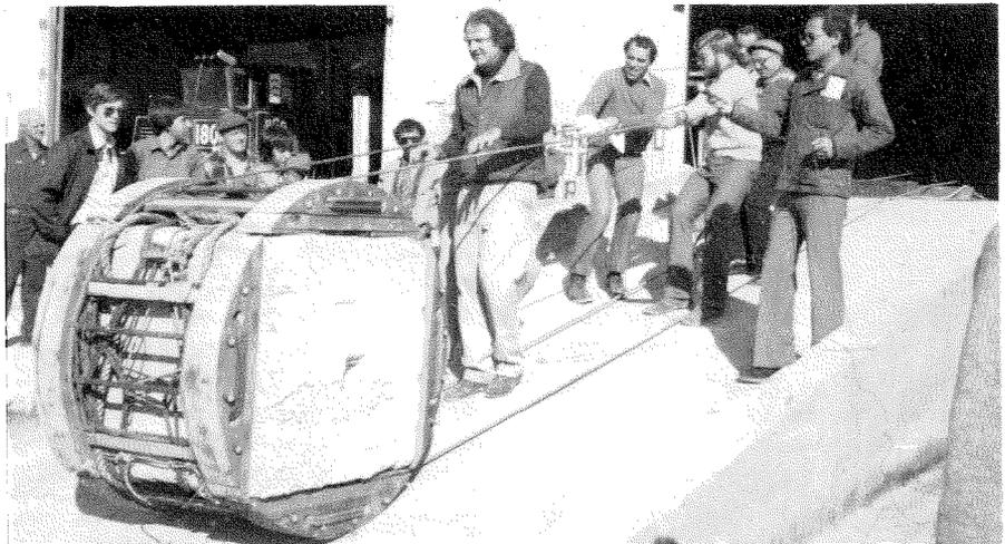
*In this photo by Linda Glick, Caltech alumnus John D. Bush (between the ropes) is demonstrating his theory that the ancient Egyptians could have built the pyramids by lashing segment-shaped cradles around blocks of stone and then parbuckling them up a ramp.*
