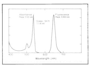
Zewail, and Cole and Amy Gupta at JPL — has discovered that a porphyrin molecule and some other similar derivatives (below, left), when incorporated into a solar concentrator, display a Stokes shift that greatly reduces self-absorption. These types of molecules are widely employed in nature as energy trappers — chlorophyll is the most important example — so Zewail believes that such molecules offer considerable promise.
