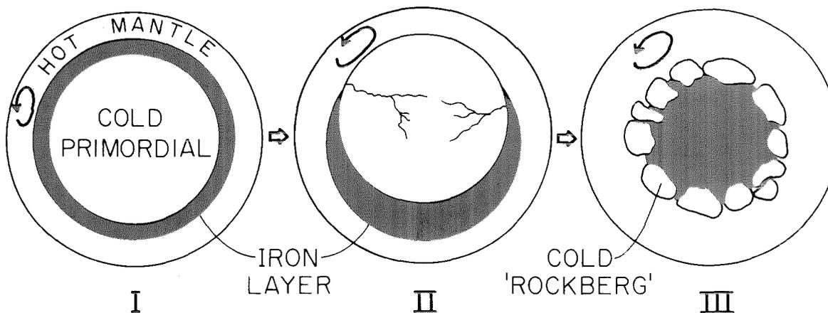
*"Catastrophic asymmetry" is one way for the heavy stuff to get to the center relatively quickly – about a million years. The central, primordial region could migrate as a rigid body through the liquid iron layer quite rapidly, creating an asymmetry that would fracture the core. The broken-up pieces of the old core – "rockbergs" – would then redistribute themselves around the new iron core.*
