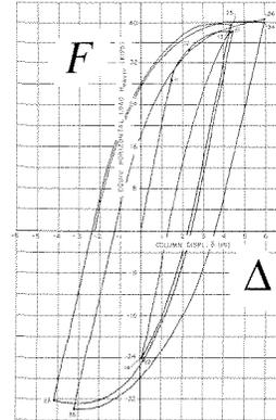
**Far right: A typical force-deflection curve from such an experiment. As in the idealized curve on the previous page, the force ( $F$ ) is plotted vertically and deflection ( $\Delta$ ) horizontally. But here the force is applied back and forth, over and over again.**
