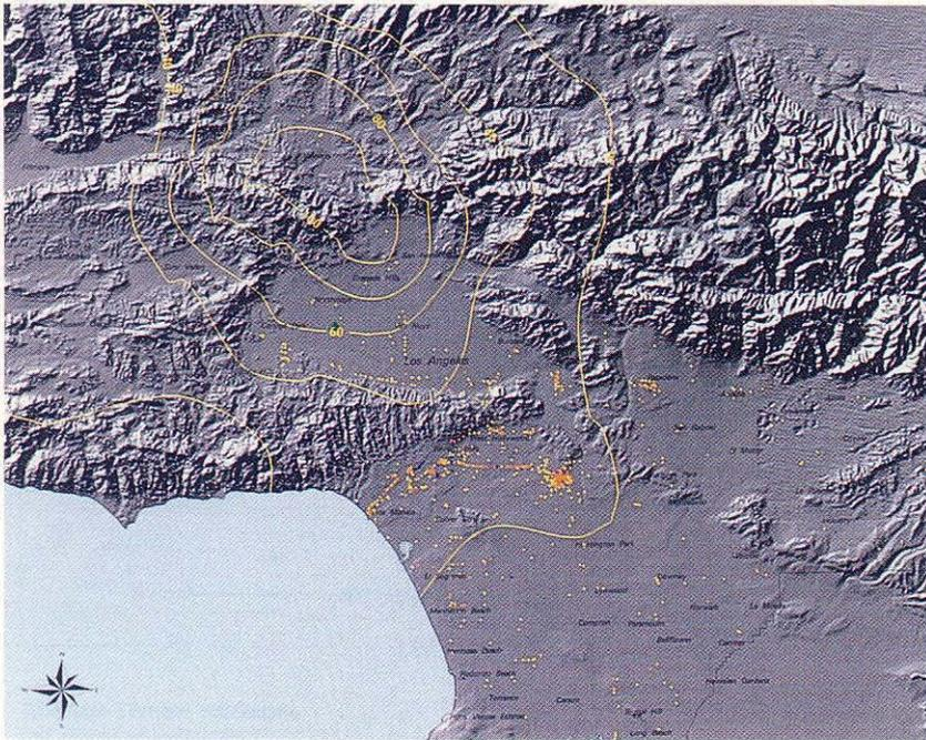
**The contours on this map of the L.A. area show peak ground velocities during the Northridge earthquake in centimeters per second. (The green triangle marks the quake's epicenter.) The dots show the locations of steel-frame buildings, as gleaned from the county assessor's records. Red dots are high-rises (six stories or taller), yellow dots are one- to five-story structures, and blue dots are buildings whose height was not recorded. Map prepared by the California Office of Emergency Services.**
