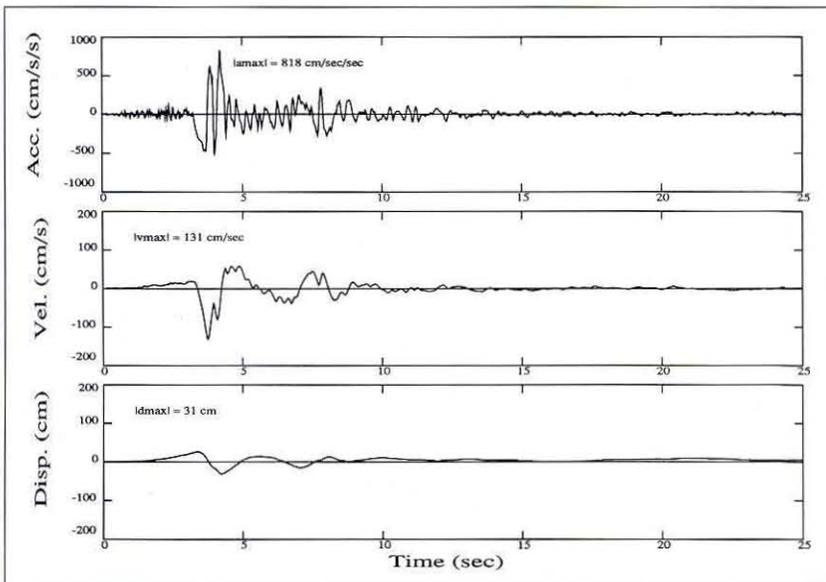
**Above:** These horizontal displacements, velocities, and accelerations (bottom, middle, and top traces, respectively) were recorded near the Olive View Hospital in Sylmar during the Northridge quake.  $l_{dmax}$  stands for peak displacement,  $l_{vmax}$  is peak velocity, and  $l_{amax}$  is peak acceleration.
