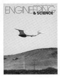
Look, up in the air — it's a . . . On the cover — a half-scale prototype (18-foot wingspan) replica of the giant pterodactyl, *Quetzal-coatlus northropi*, glides above Simi Valley in a radio-controlled test flight last August. This model was used to develop the lateral-control autopilot. The streamers trailing behind serve to indicate air flow to observers on the ground.
